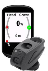
measure the chest and headheight and it gives the cyclist instant, real-time feedback on their bike computer to assist them with maintaining their optimal aerodynamic position. Streamlines was launched in 2021 to further simplify and improve the user experience of aerodynamic testing, including the refinement of the FORMA sensor before bringing it to market."
